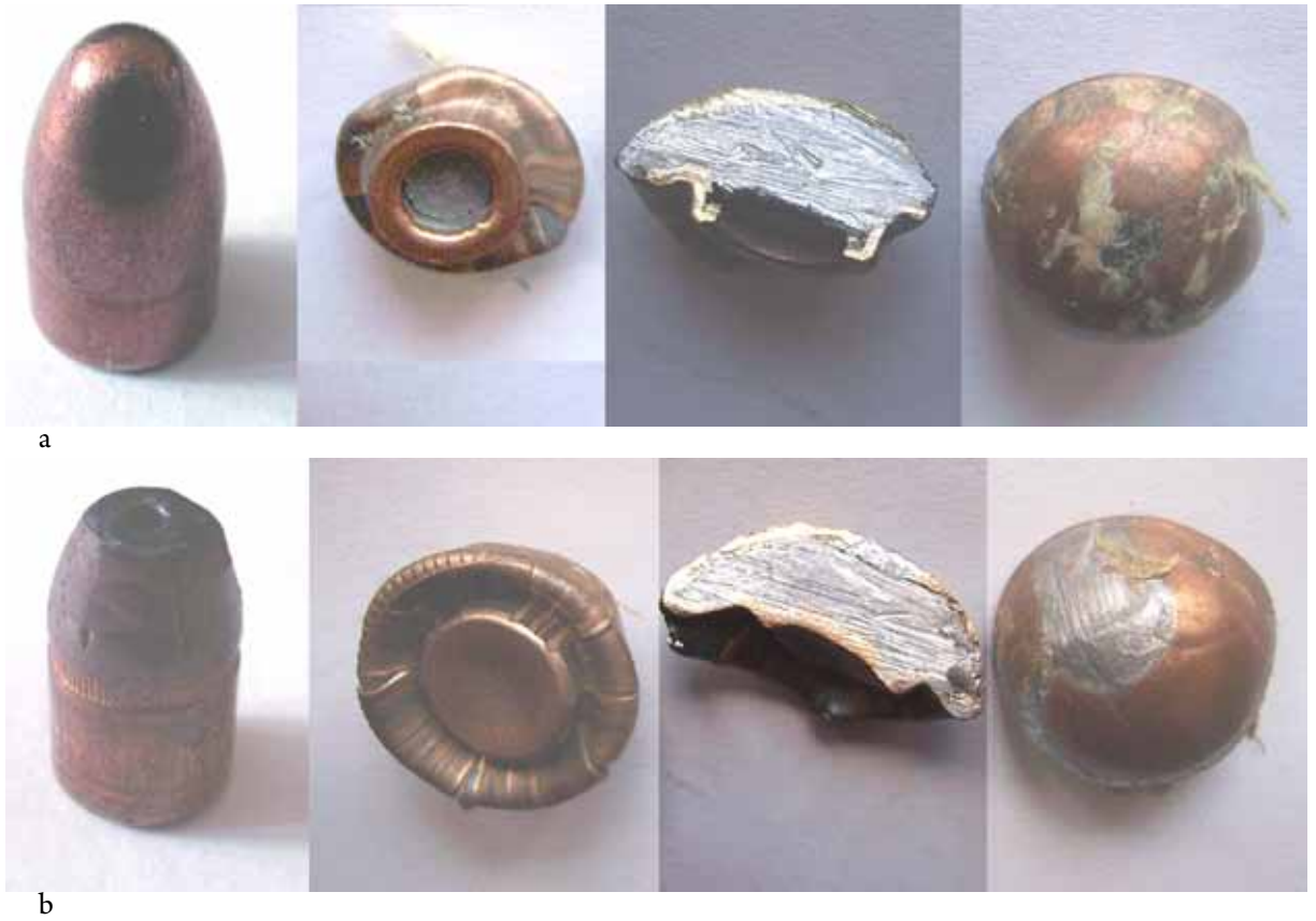
Fig.2: Lead bullets after interaction with textile armor a) [top] FMJ 9mm Parabellum b) [bottom] JHP 0.44 Magnum
