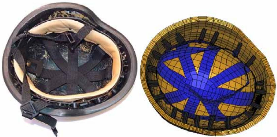
*Fig. 1. Helmet's interior and its FEM model, used for simulations [19].*
