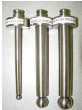
Figure no 3 - Pins with balls, from the left diameters: Ø10, Ø20, Ø25.4 mm respectively
